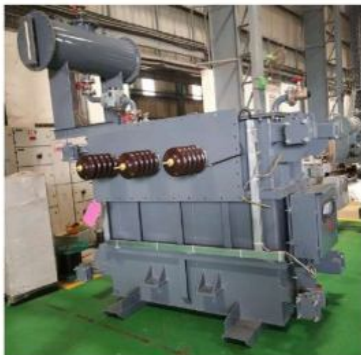
3MVA, 33/433v OCTC Transformer for M/s. Indorama, Nigeria
